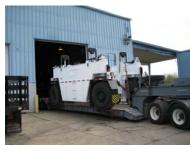
Operator's Cabin is **Easily Removed for** Transport on Standard Low Boy Trailer.
