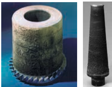
Both of these filters look ready for replacement, but neither have reached their final servicing point.
