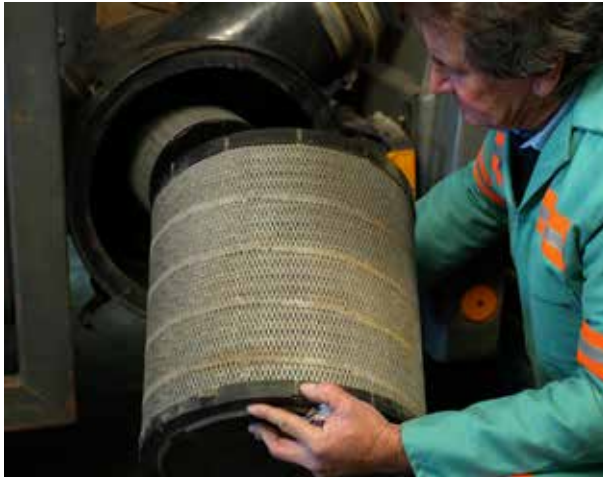
Although this air filter may look "dirty" — it can go plenty more miles. Installation of a restriction indicator can save you money and time.
