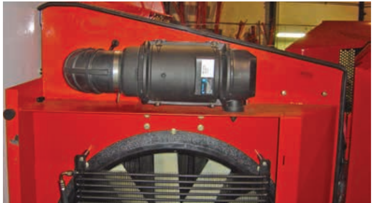
A PSD10 mounted horizontally was the equipment manufacturer's choice on this diesel-powered (285 HP @ 2,000 RPM) feller buncher.
