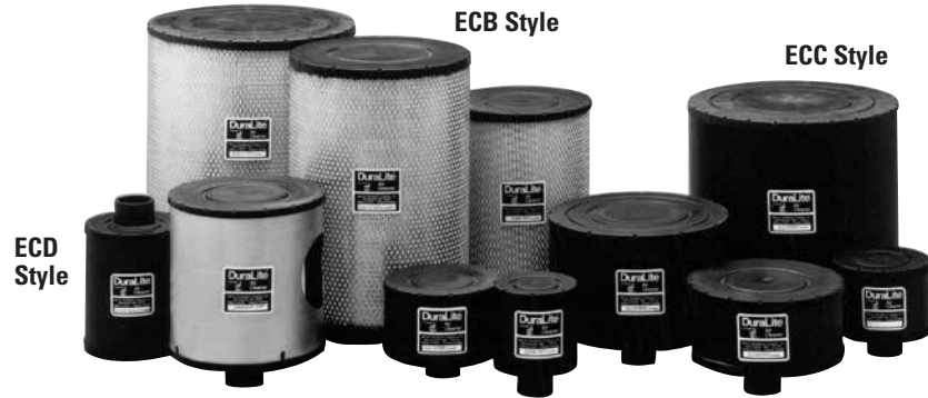
DuraLite™ Air Cleaners — sturdy, one-piece, and disposable — are designed to withstand the high pulsation of small engines such as the ones shown here. They are easy to maintain because there are no service parts. When the filter is full, simply throw it away.
