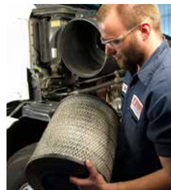
The clean side of your air filter can vary depending on the application. Some filters load on the outer surface (shown above — referred to as standard flow), and some load on the inside surfaces of the filter (referred to as reverse flow).
